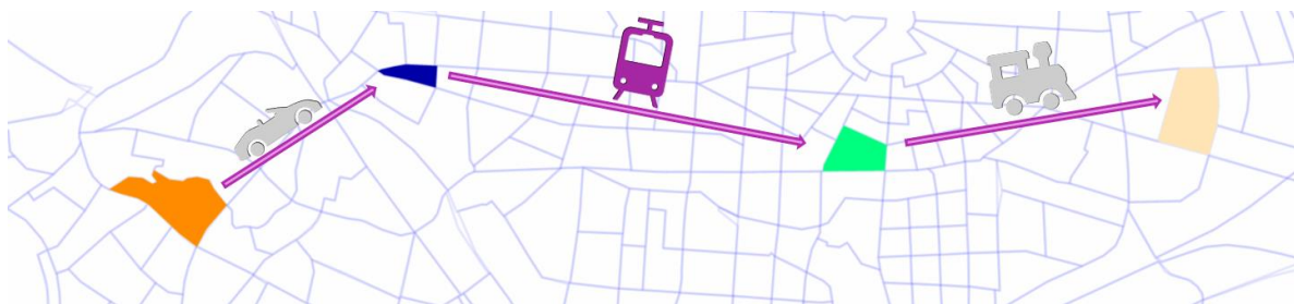
Figure 4: The intermodal assignment combines multiple modes within a single trip. There is always one mandatory mode and one or more optional feeder modes. Transfers occur at zones.
